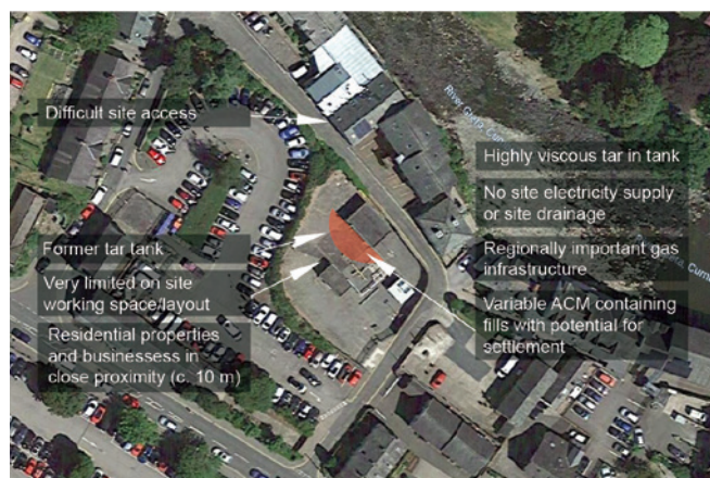
Figure 2 - Summary of constraints to remediation at Keswick Gas Site
